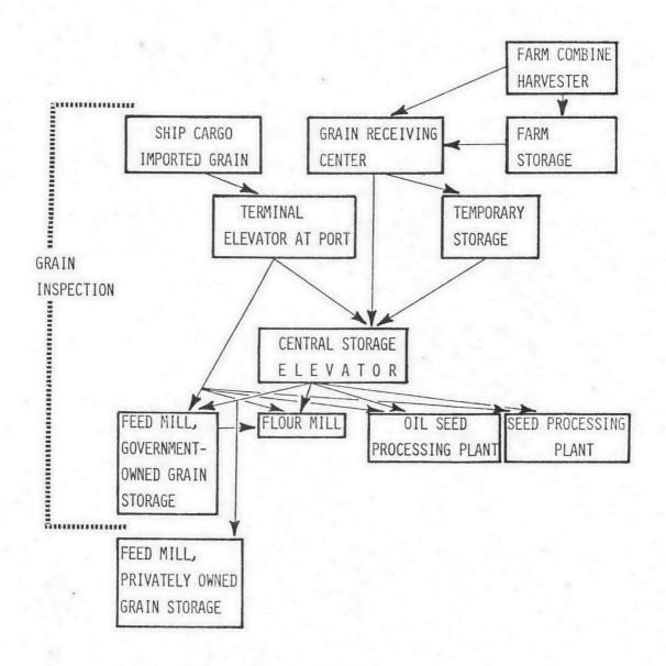
Fig. 2 - Commodity flow diagram showing different stages of storage.
