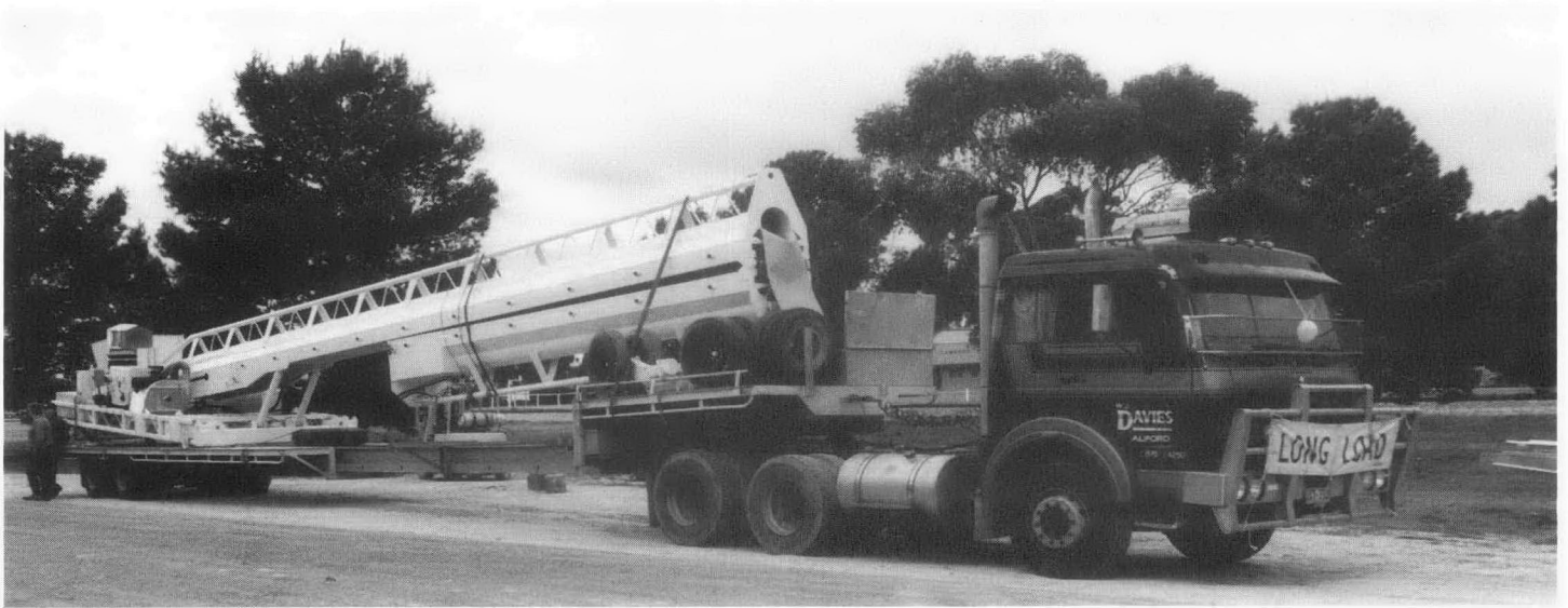
Fig. 5. Extendable trailer carrying tube assembly.
