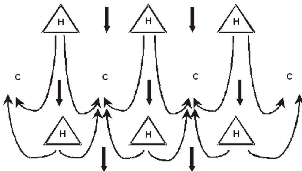
**Figure 4.** Schematic diagram of a mixed-flow dryer. Thicker arrows indicate grain flow, thinner arrows airflow, H hot air duct, and C exhaust air duct.
