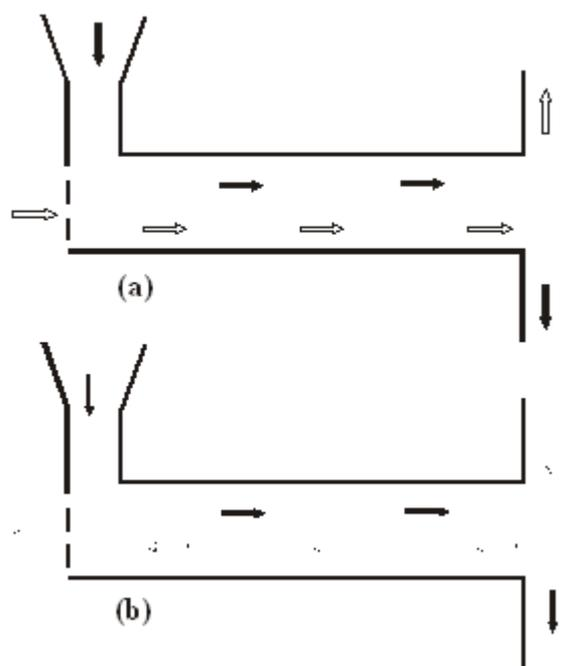
**Figure 3.** Schematic diagrams of different dryer designs; (a) concurrent-flow dryer, (b) countercurrent-flow dryer (refer to Figure 2 for description of arrows).
