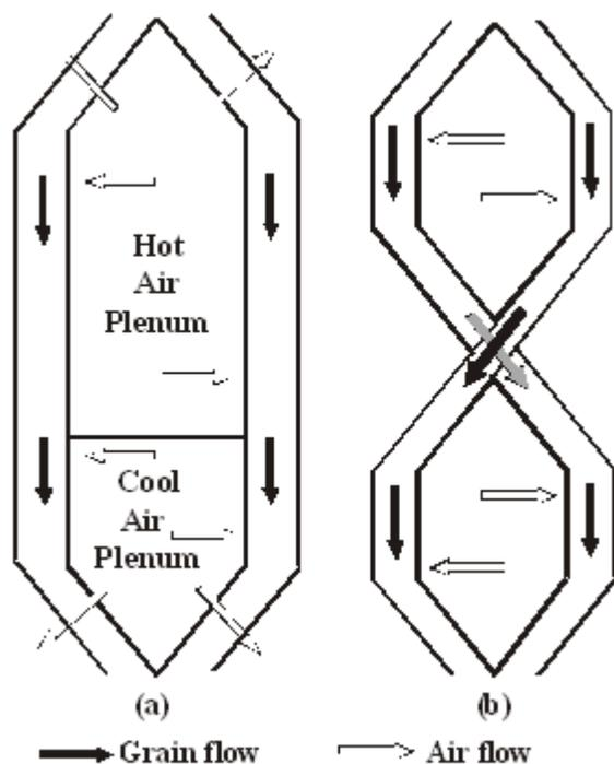
**Figure 2.** Schematic diagrams of different dryer designs; (a) cross-flow dryer, (b) Sukup double cross-over flow dryer.
